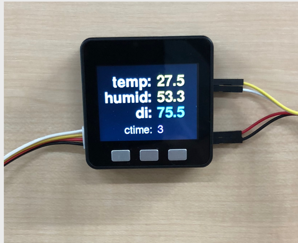
M5 Stack (CPU: ESP32 240MHz, Flash: 16MB, RAM: 520KB)
